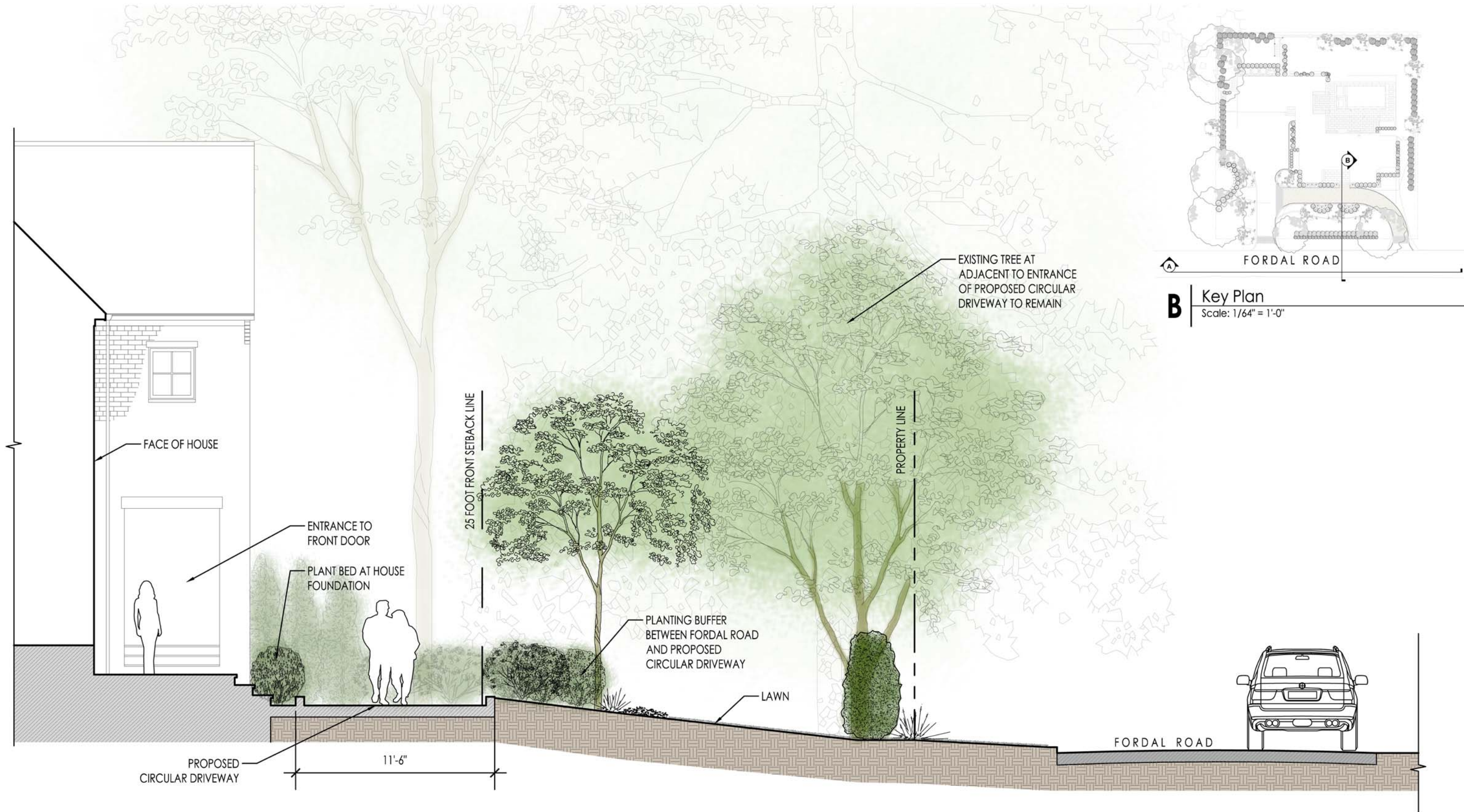
2 Section B - Section Cut from Fordal Road Through to Front Entrance Scale: 3/16" = 1'-0"
