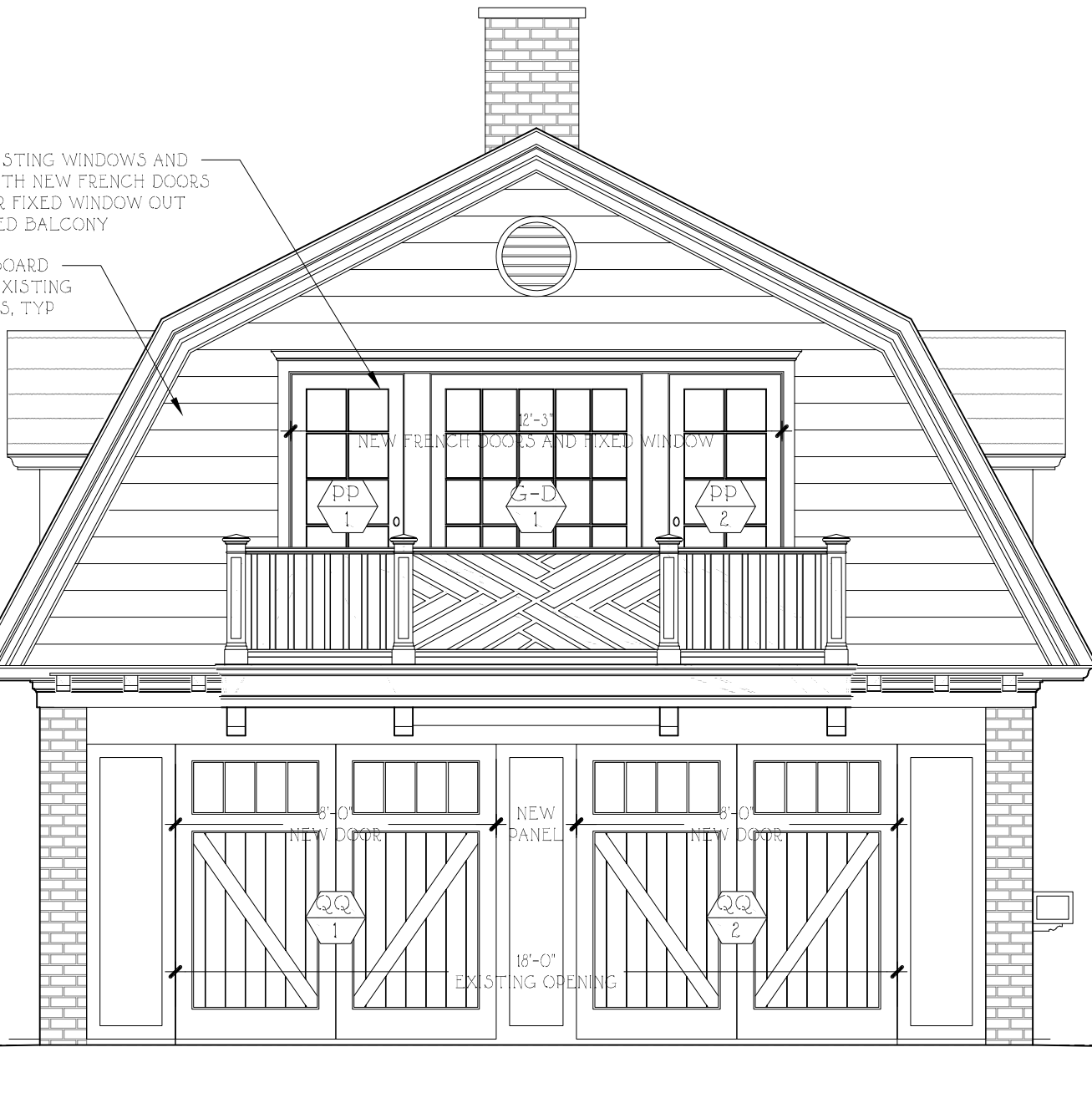
4 CARRIAGE HOUSE - WEST ELEVATION 1/4"=1'-0"
